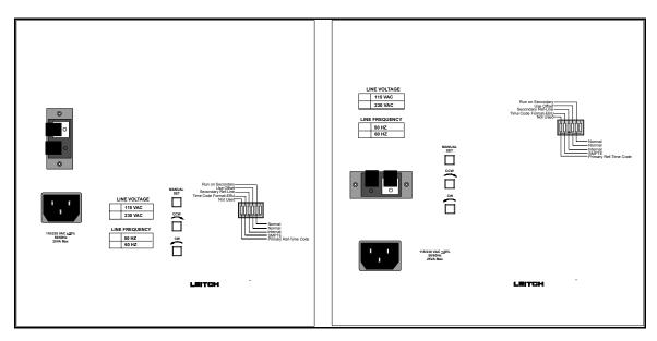
Figure 1-3. DAC-5005 (left) and DAC-5006 (right) Rear Panels
