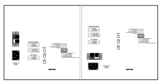
Figure 2-6. ADC-5105 (left) and ADC-5106 (right) Rear Panels
