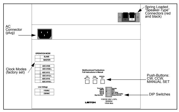
Figure 2-5. ADC-5108/5112/5116 Rear Panel
