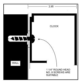
Figure 2-4. Typical Wall Mounting
