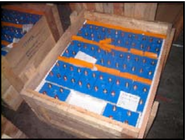
NiFe batteries shown in their shipping crates, with orange battery post covers to meet NEC requierments.
