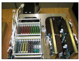
Node boards have a Euroboard 3U form factor (100 cm x 160 cm) and are typically mounted in 9-slot HIDAS Backplanes installed in 3U VME/Euroboard racks. Backplanes are passive boards that simplify mounting, data link connections, and power distribution. Backplane and rack configuration can be custom or can be configured 3 Backplanes across (27 Node boards) to mount in standard 19-inch (48.26 cm) racks.
