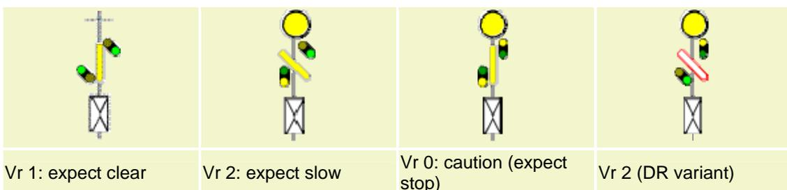
The rectangular sign at the signal's post is the distant signal post plate. indicates its position, so it will be clearly visible when the disc is flipped edge-on.
