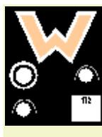
This is a device combining a Ra 11 Waiting board a Ra 12 light signal and often a Kreisscheibe (Circle Board). The white box at the lower right contains the signal's number. The "W" is transparently illuminated. If the two white lights are off it means 'stopping for shunting movements', see also Ra 11. If they are on, they are an order to proceed (without the Kreisscheibe it would be just a permission).
