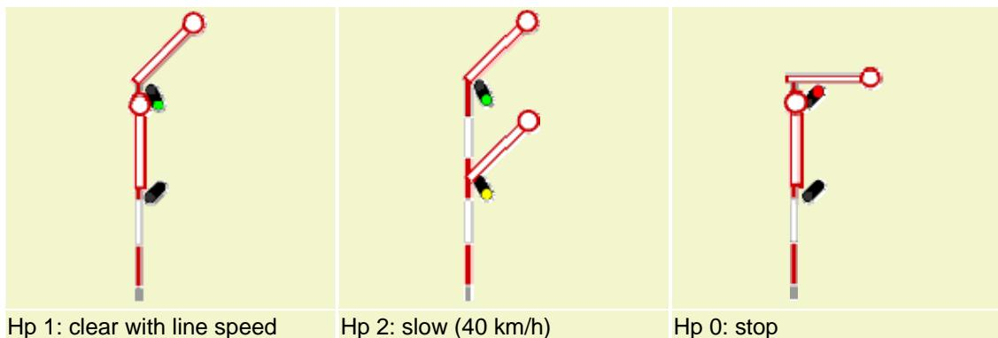
The signals are also equipped with lanterns that are lit at night, by gas lanterns in the old days, now by solar-driven LED matrices.
