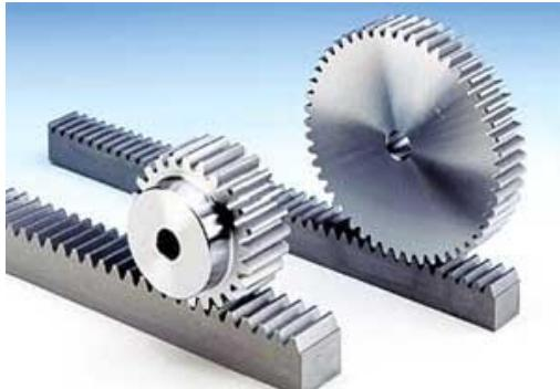
Standard metric spur gears and rack available from stock in non-hardened form. Rack and pinion is a traditional drive system that provides a compact and rugged linear or geared drive. Standard racks are 2m long and can be butt joined for an unlimited length. A great benefit of rack and pinion is its high rigidity even in very long length applications. It is also easy to install and can operate at high speed.
