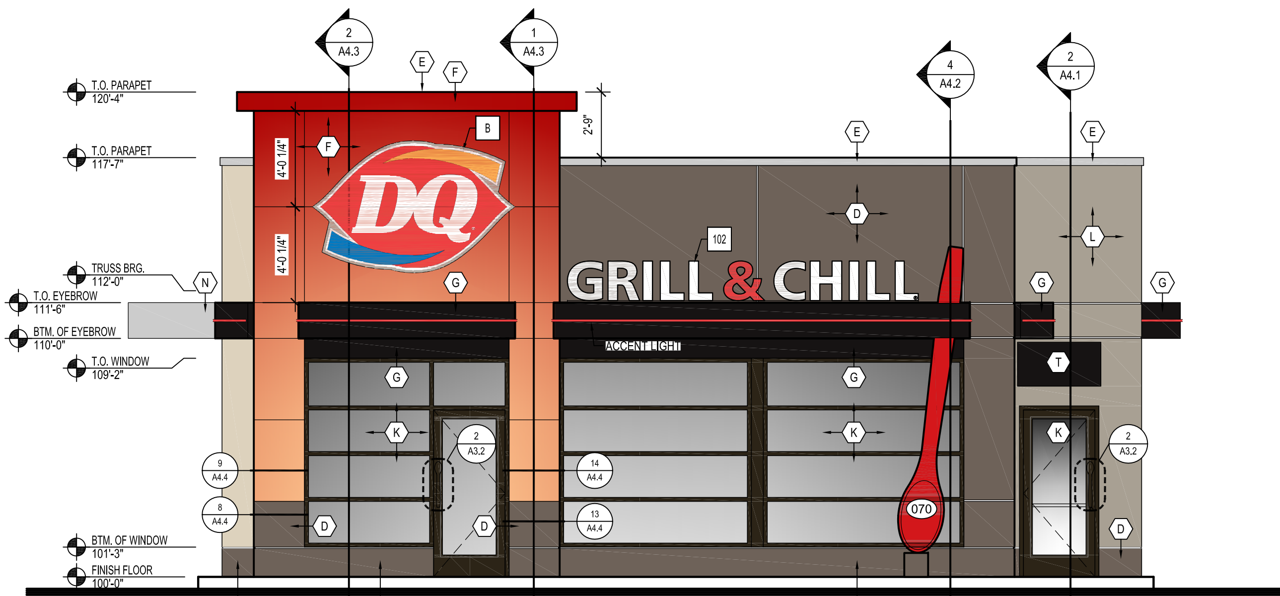
1 FRONT ELEVATION A3.1 SCALE: 1/4" = 1'-0" NOTE: THE DO RED SPOON HANDLES HAVE SPECIAL INSTALLATION REQUIREMENTS. ALUM. STOREFRONT MFG. MUST COORD. LOCK & HANDLE, LOCATION & HEIGHTS
