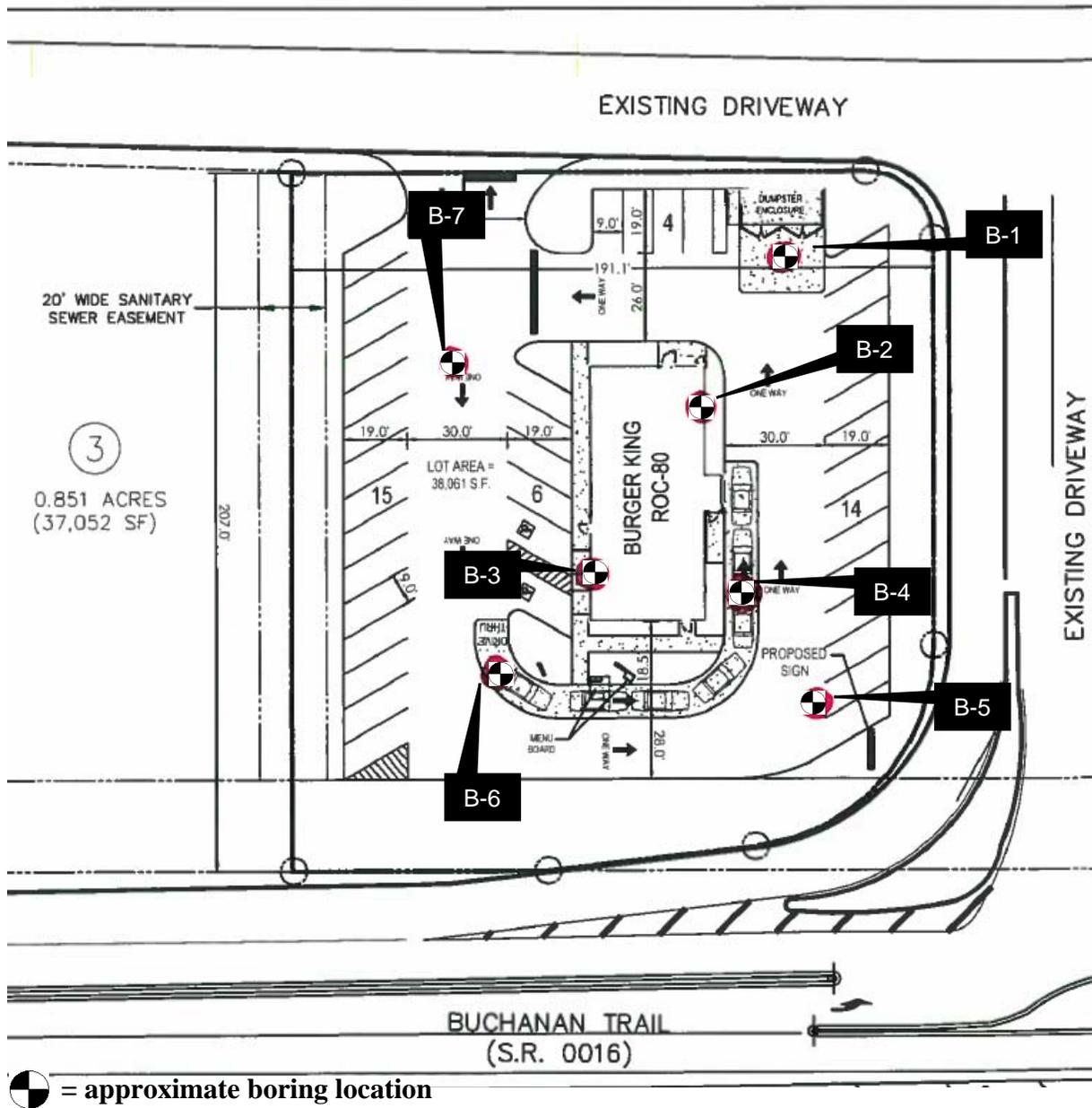
**Figure 1 Field Work Location Plan**
