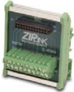
ZL-RTB20 20-pin feed-through connector module
