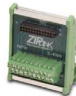
ZL-RTB20 20-pin feed-through connector module
