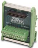
ZL-RTB20 20-pin feed-through connector module
