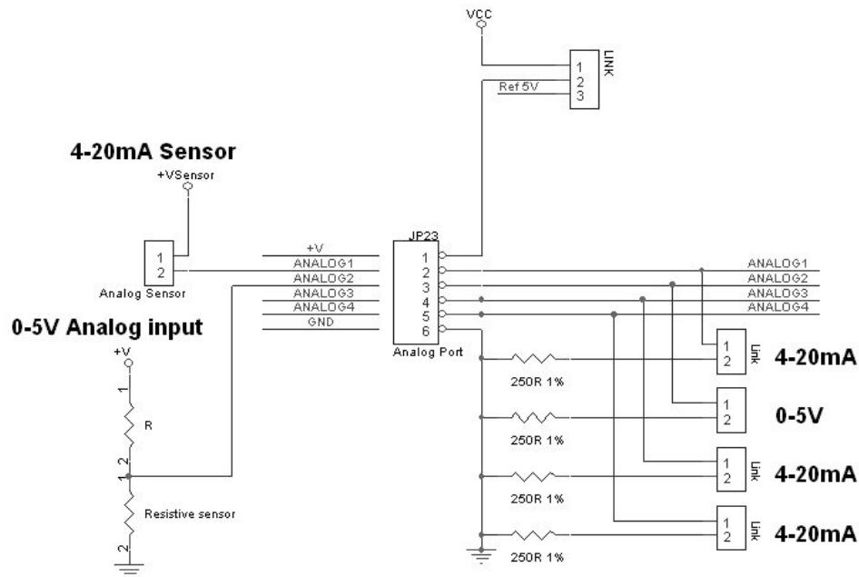
The analog input can be either 0-20mA or 0-5V. If the link is connected the 0-20mA option is selected. The 250 ohm resistor will convert the 0-20mA to a voltage of 0-5V. The communicator use a 10 bit A/D converter and the value of 0-5V will correspond to a value of 0-1023 in the communicator.
