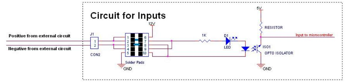
No common supply. Positive and negative is supplied from external alarm circuitry.
