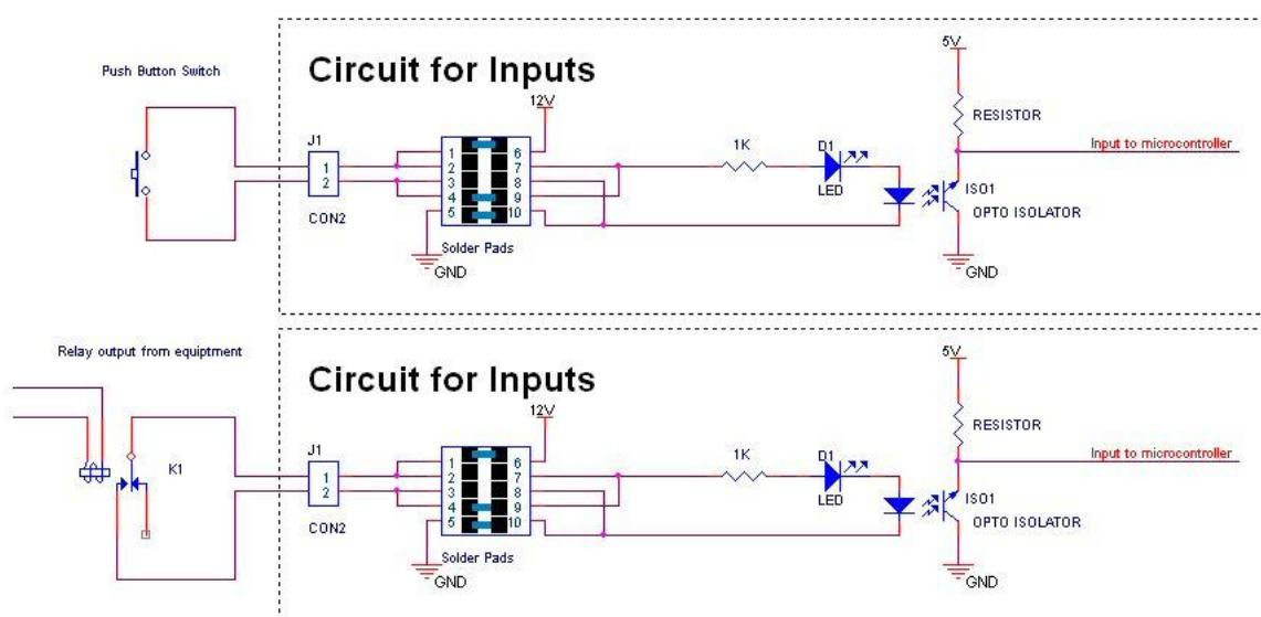
If the switches are closed the corresponding Input will go on and SMS will be send to the configured telephone numbers.
