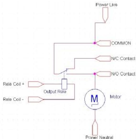
Output used to switch on a motor using less than 240VAC and 10A current
