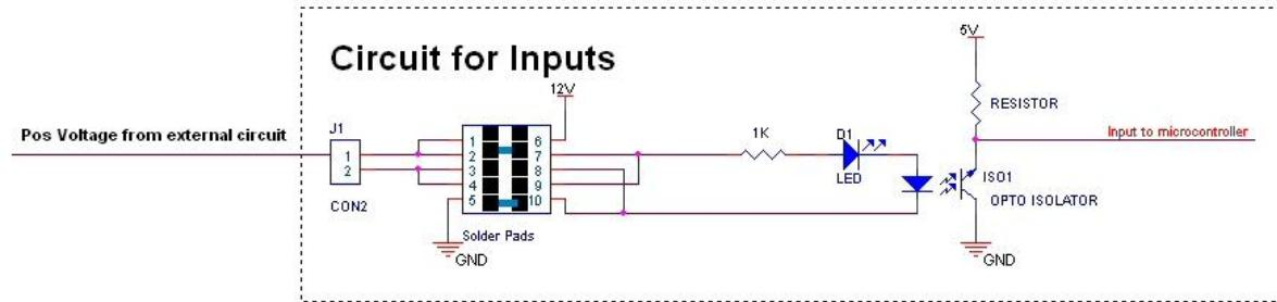
If a common supply is used then a positive from the alarm circuit can be used to trigger the unit.
