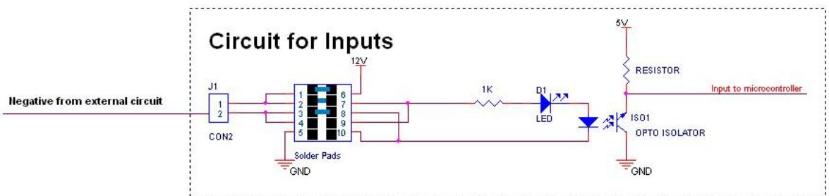
If a common supply is used then a negative from the alarm circuit can be used to trigger the unit.
