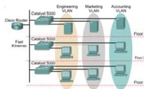
VLANs logically segment switched networks based on an organization's functions, project teams, or applications as opposed to a physical or geographical basis.
