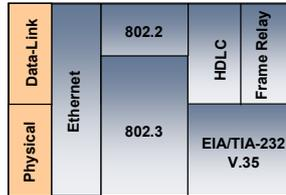
LLC: The upper component of the data-link layer that provides data repackaging functions for operations between different network types.
