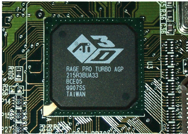
FIGURE 2.15 Markings on chips can help identify the chipset for XFree86.
