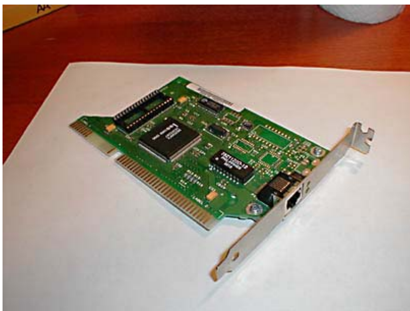
Figure 17.13 An Ethernet NIC that uses an RJ45 jack
