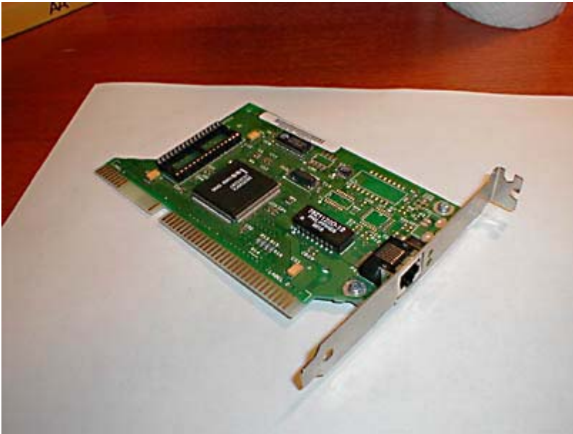
Figure 2.7 Network interface adapters usually take the form of expansion cards.
