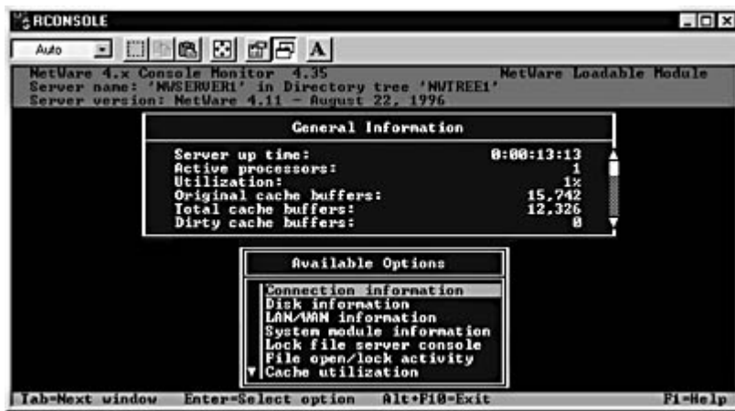
Figure 4.3 The NetWare server console is character-based, but uses keyboard-driven menus.
