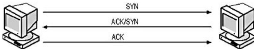
Figure 7.2 TCP uses a three-way handshake to establish a connection between two systems.
