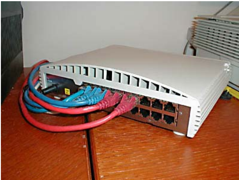
Figure 2.10 Hubs have ports into which you plug the cables connected to your computers' network interface adapters.
