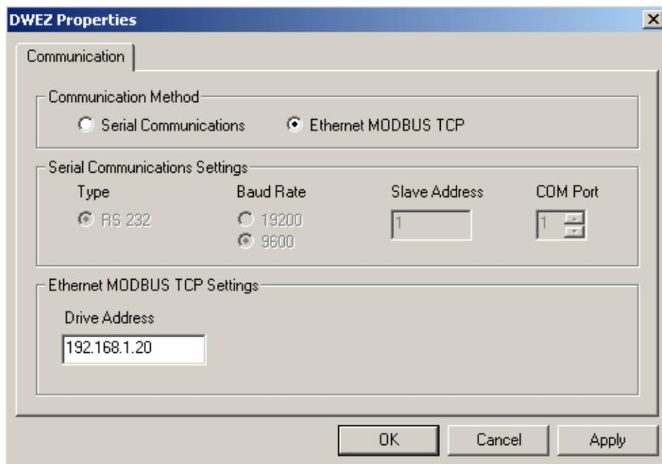
Change *Communication Method* to *Ethernet MODBUS TCP* and type in the IP address of the G7 drive in the *Drive Address* box. Click *OK*. Use this setting for the CM092 EtherNet/IP kit as well.
