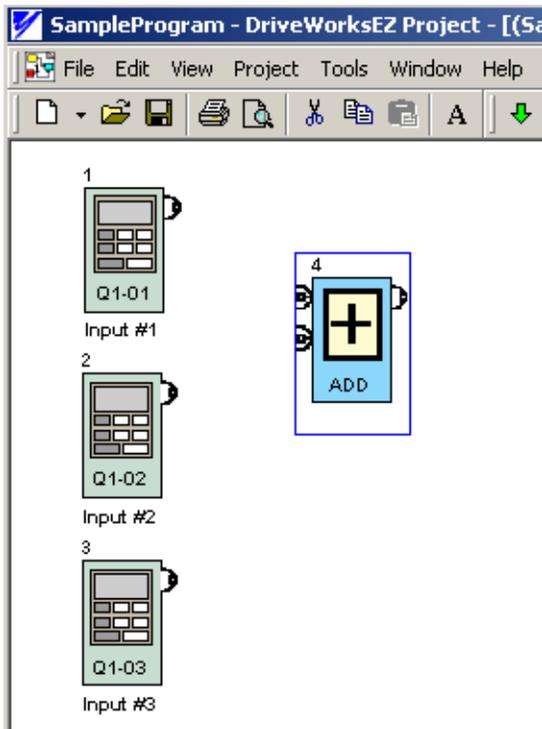
9. To make the first connection, position the cursor over the numeric output node of the Q1-01 block. Click and hold the left mouse button and move the cursor towards the numeric input upper node of the ADD block. A short line will be noticed on the output node indicating that the PC Tool is in the line draw mode. The PC Tool will automatically finish the connection, so the left mouse button can be released. A placeholder for the monitor value will display the current value of that connection.
