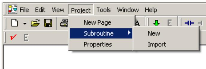
A new subroutine can be created by selecting the *Project* pull-down menu and selecting *Subroutine* and then *New*. The name given to the subroutine will also be the name used for the subroutine file saved in the project folder.
