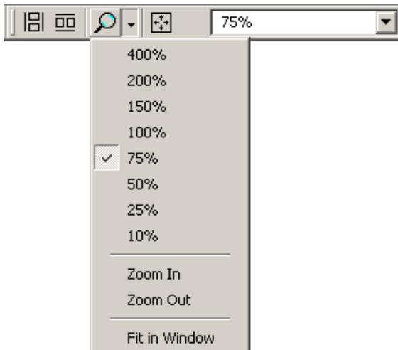
**Fit In Window** – Adjusts to the zoom level so all of the blocks will fit in the window.
