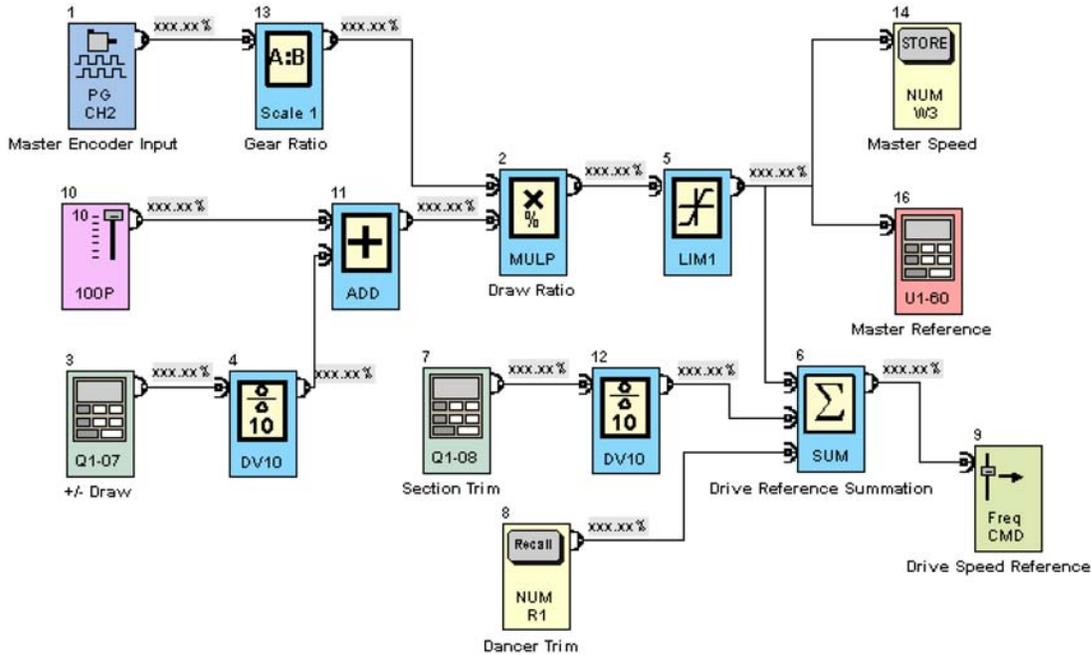
The master encoder speed comes into the program in block 1(PG CH2). The parameter setting of Q2-02 along with the settings of block 13(Scale 1) that are parameters Q4-03, 04, 05 are adjusted to derive a value of 100.00% at the output of block 13(Scale 1) when the master device is at 100% of its speed.
