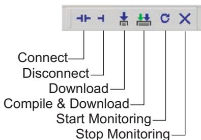
**Connect** – Establishes communication with drive per DriveWorksEZ™ Properties settings provided the drive is set for DriveWorksEZ™ access.
