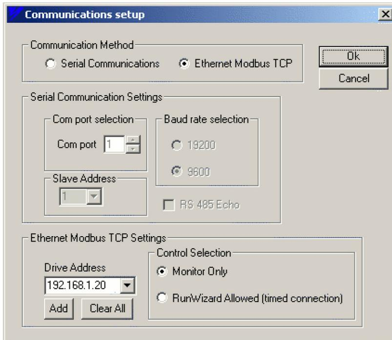
Change *Communication Method* to *Ethernet Modbus TCP* and type in the IP address of the G7 drive in the *Drive Address* box. Click *OK*. Use this setting for the CM092 EtherNet/IP kit as well.
