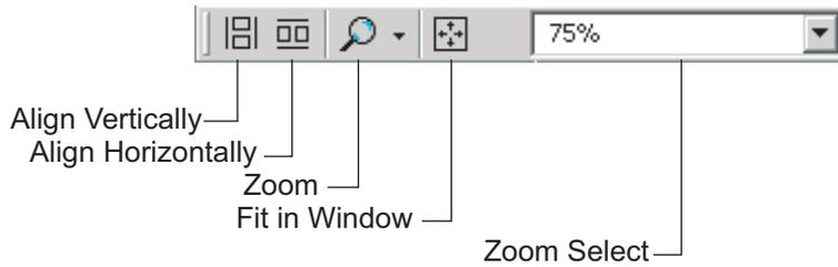
**Align Vertically** – This tool vertically aligns the highlighted blocks. It will only be enabled if more than one block is highlighted.
