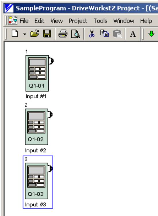
8. Add the math functions to the program. Select the *Numeric Function* tab on the *Block Toolbar* and drag the ADD block onto the page to the right of the Q1-01 and Q1-02 blocks.
