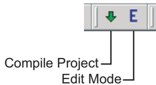
**Compile Project Mode** – Takes the pages of the open project and checks the connections for errors and then translates the project into a connection list.
