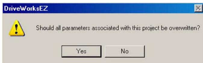
Another solution to prevent incorrect operation of the DriveWorksEZ™ programming due to a drive initialization is to save the settings of the standard parameters with a User Default save (o2-03=1). See the *Precautions* section after the first successful operation of the DriveWorksEZ™ program.
