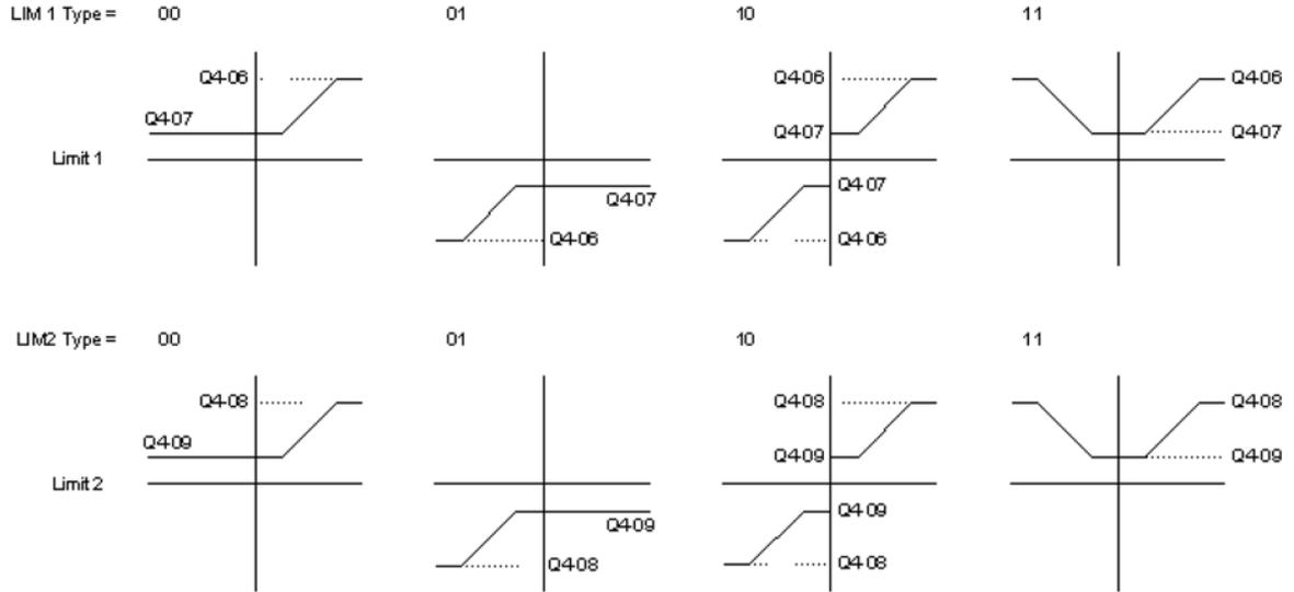
DZONE is used to zero data when it is below the set Dead Zone (Q4-10) value. DZONE can be positive, negative, bipolar, or absolute value and of type A or B, as shown below.
