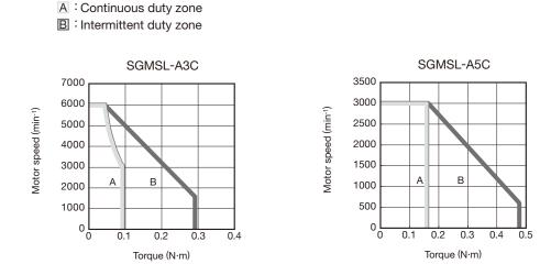
Note: 1. These values are for operation in combination with a SERVOPACK when the temperature of the armature winding is 100°C. These are typical values. 2. The characteristics in the intermittent duty zone depend on the power supply voltage.
