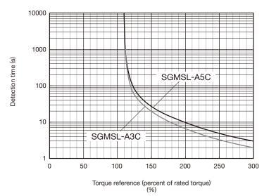
Note: The above overload protection characteristics do not mean that you can perform continuous duty operation with an output of 100% or higher. Use the Servomotor so that the effective torque remains within the continuous duty zone given in *Torque-Motor Speed Characteristics*.
