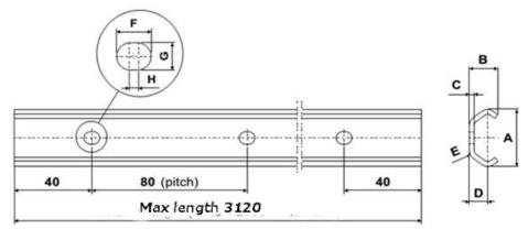
Recommended fastener is a button head cap screw
