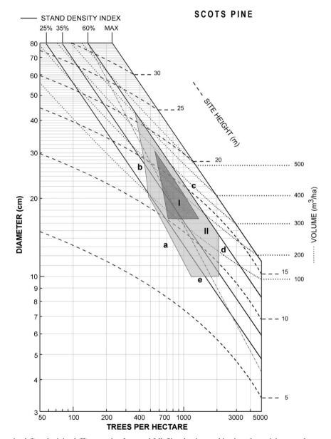
Fig. 6. Suitability zone for optimal (I) and minimal (II) protection from rockfall. Size-density combinations determining complete canopy closure (dash and dotted line) are superimposed on the DMD. Suitability zones are defined by (a) minimum crown closure; (b) minimum MTFD; (c) minimum crown ratio; (d) maximum tree slenderness; (e) minimum QMD.
