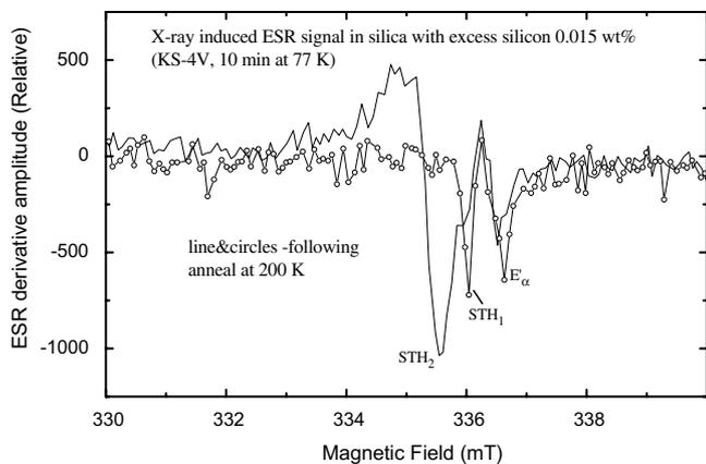
Fig. 3. X-ray-induced ESR signals in KS-4 V silica with excess silicon 0.015 wt% at 77 K. Line without symbols: immediately following irradiation without warming. Lines & circles: following anneal at 200 K.
