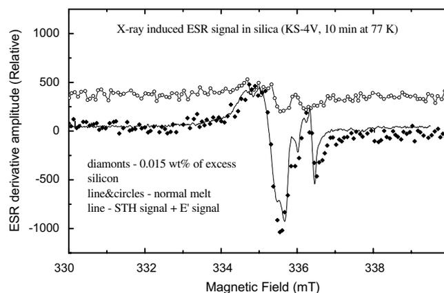
Fig. 2. X-ray-induced ESR signals in KS-4 V silica at 77 K. Diamonds: silica doped with 0.015 wt% of excess silicon. Lines and circles: normal stoichiometric melt. Line without symbols: ESR signal for a Suprasil W1 fused silica sample exposed to X-rays at 77 K and recorded at 110 K (from Ref. [13]).
