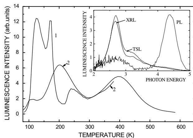
Fig. 1. Thermally stimulated luminescence (TSL) in KS-4 V silica with excess silicon (0.015 wt%) recorded at 2.7 eV after irradiation by X-rays (curve 1) and 7.7 eV photons (curve 2) at 77 K. Inset: luminescence spectra of samples of the same material continuously excited by X-rays (XRL) and by 7.7 eV photons (PL) with comparison to the spectrum of the TSL. The temperature was  $\sim 80$  K for XRL and PL and  $\sim 120$  K for TSL.
