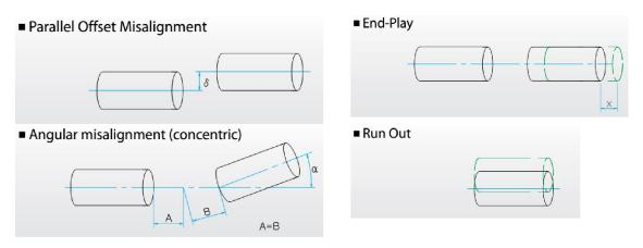
If there is no misalignment ability in the coupling then moment loads will be generated between the two shafts and this load will cycle with every rotation of the shaft. When shafts are in constant motion or at high speeds then what we end up with is a perfect configuration to create fatigue failure of the shaft itself. In cases of high misalignment inaccuracy of motion and vibration of the mechanism can occur.
